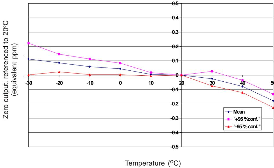
Figure 2 shows the variation in zero output caused by changes in temperature expressed as ppm gas equivalent.
